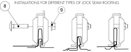
Tighten the bolts of the fastener until the apparent elastic limit, i.e. until the sides of the fastener have come closer to each other but have not become dented or twisted.
