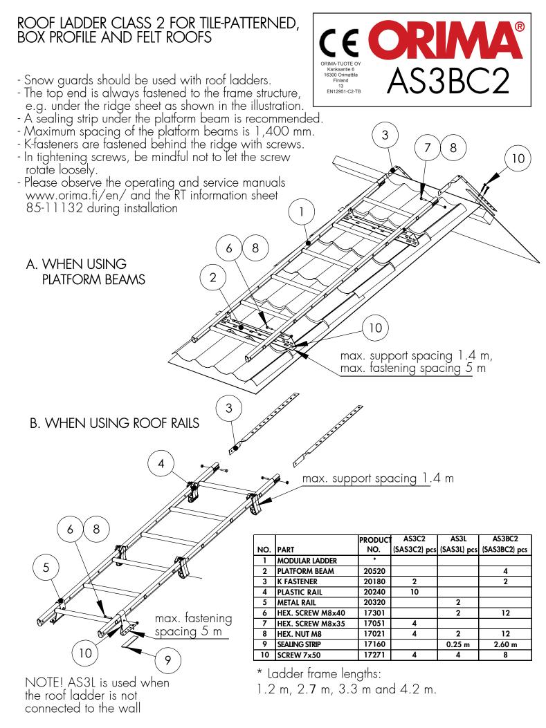
NOTE! The screw strength M8 8.8(ISO 898) must be used.
